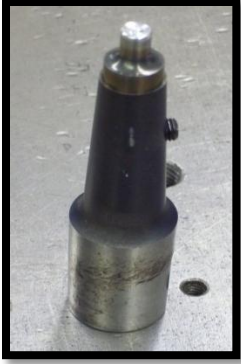
Figure 4. Pin used for welding.
